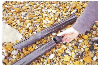
ABOVE The 10.2sq m mainsail requires an additional 350mm stub to the two-piece carbon rig.
