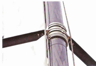
ABOVE The whole mast rotates inside a custom spreader bracket: spreader angle is fixed, but length adjustable.
