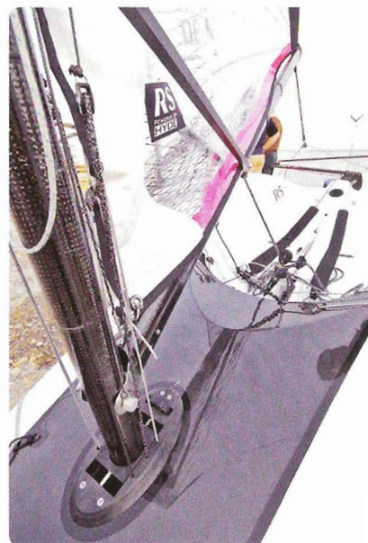
ABOVE The carbon foredeck adds stiffness and forms the top of the spinnaker chute.
